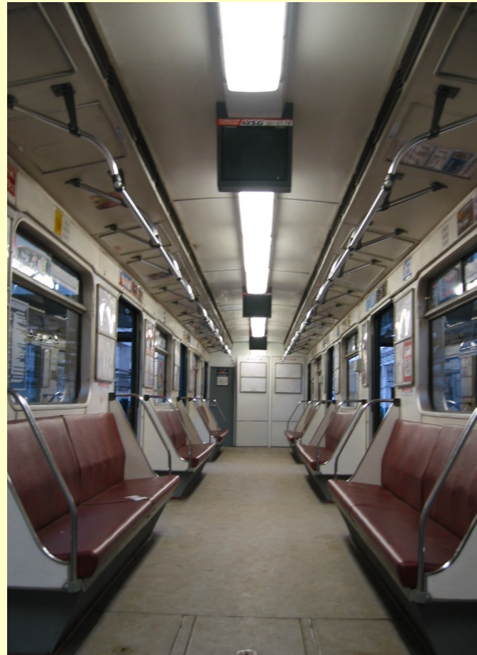
Subway car 81-717 series is equipped with the LED lamps
